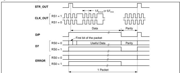
Figure 7: Parallel Output Interface
